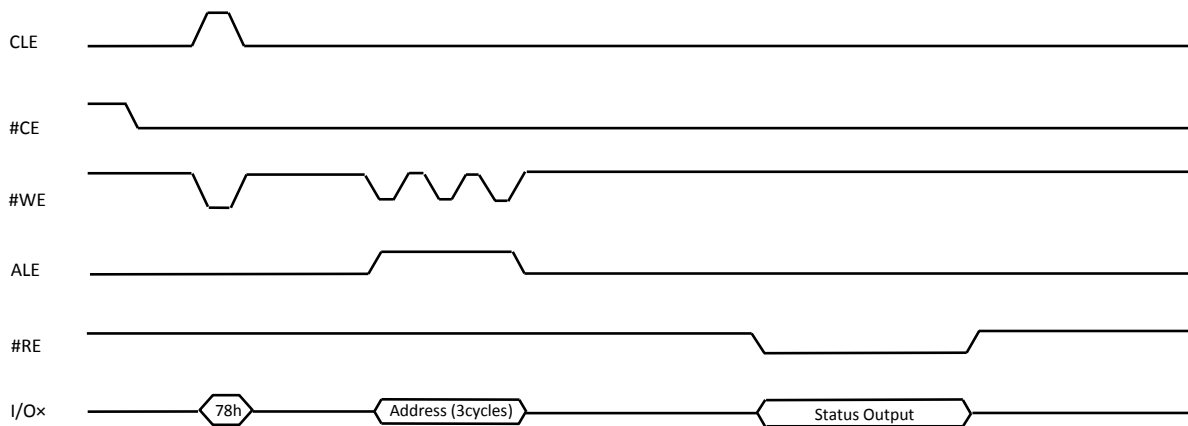
Figure 9-11 Read Status Enhanced (78h) Operation
